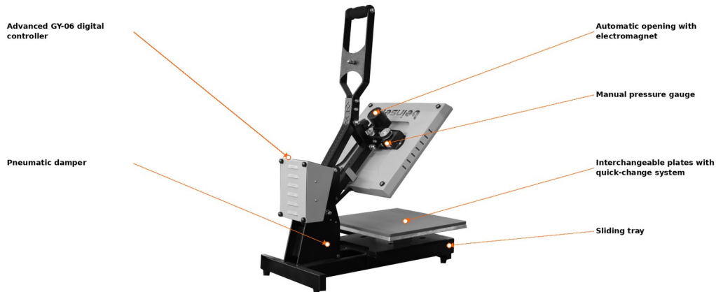
Fig. 1 · Main components of the Beinsen Barbados.
