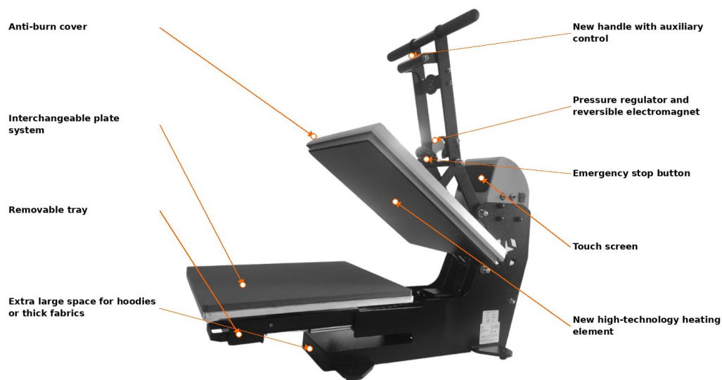
Fig. 1 · Main components of the Beinsen Malvinas.
